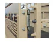
standard vehicle. When in transport mode, the cage is locked down to the frame. This prevents cage movement and load cell damage during transport.
